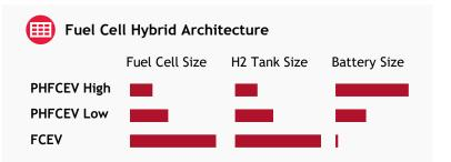
Some highly intensive use of passenger cars such as taxis are now the focus of fuel cell technology. Similarly, light commercial vehicles need high range and have to carry heavy loads requiring a large, heavy and costly battery. For these type of vehicles there is a case for fuel cell technology that has an advantage on range and can allow higher power output with a powerful fuel cell stack. However, there is a large hydrogen tank that can not be reduced despite developing high pressure vessels.
